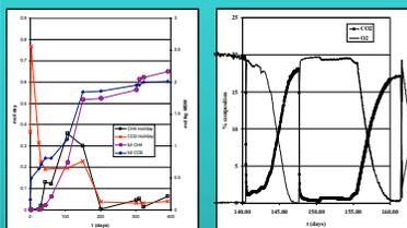
Landfill gas composition from the anaerobic, wet tanks
